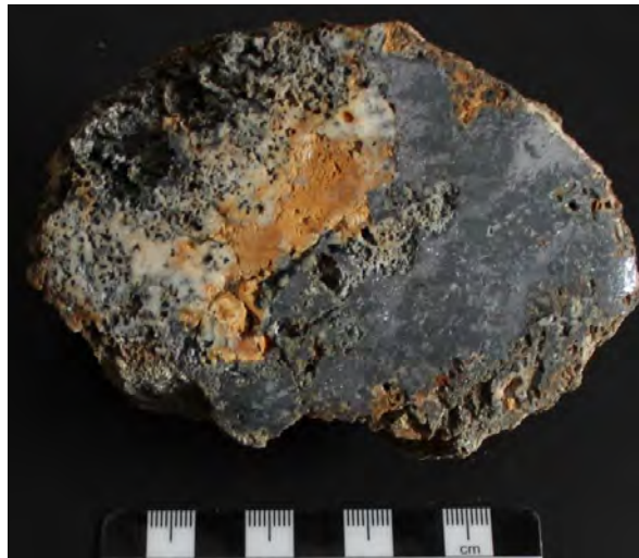
Golden Lion Photo 6: GL1 Target Area, Zone 2 epithermal style mineralization: 2017 sample no. D005160: quartz vein hosting semi-massive galena, sphalerite +/- sulfosalts; 1,545 g/t Ag, 16.7% Pb, 1.1 g/t Au (A. Albano, 2018)
