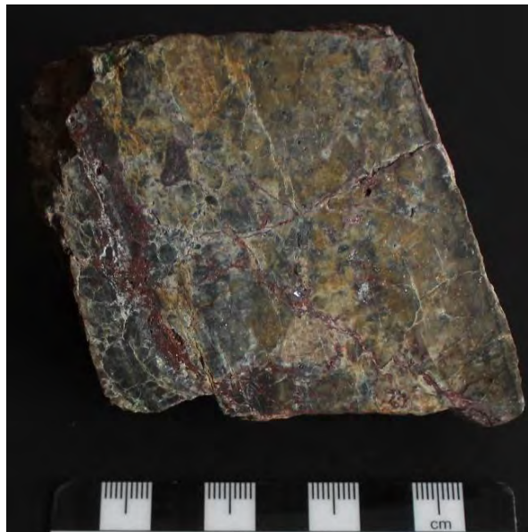
Golden Lion Photo 7: GL1 Target Area, Zone 2 epithermal style mineralization: sample no. D005158: quartz vein hosting semi massive galena, sphalerite +/- sulfosalts; 2,640 g/t Ag, 1.18% Pb (A. Albano, 2018)
