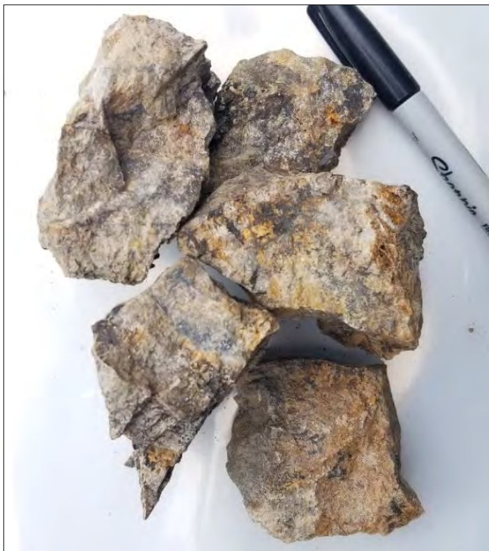
Golden Lion Photo 18: Sample T19GL1F-03: Potassic altered felspar intrusive (monzonite?) with boxwork textured quartz veining and minor galena. Dendritic manganese is common on fractures (D. Tupper, 2019)
