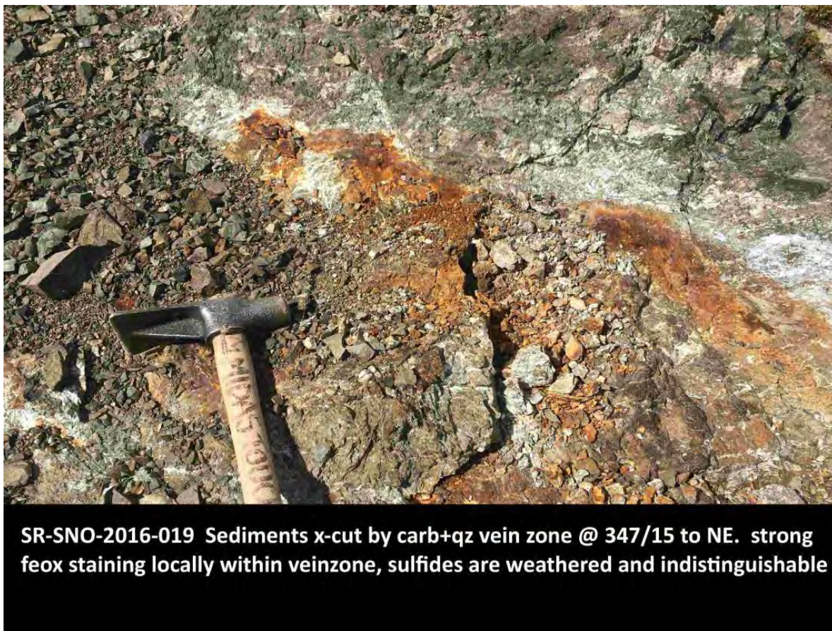
Photo 18. Sheeted veins or stockworks at Snoball have potential for wide zones of low to moderate grade gold and silver (C. Greig, 2016)
