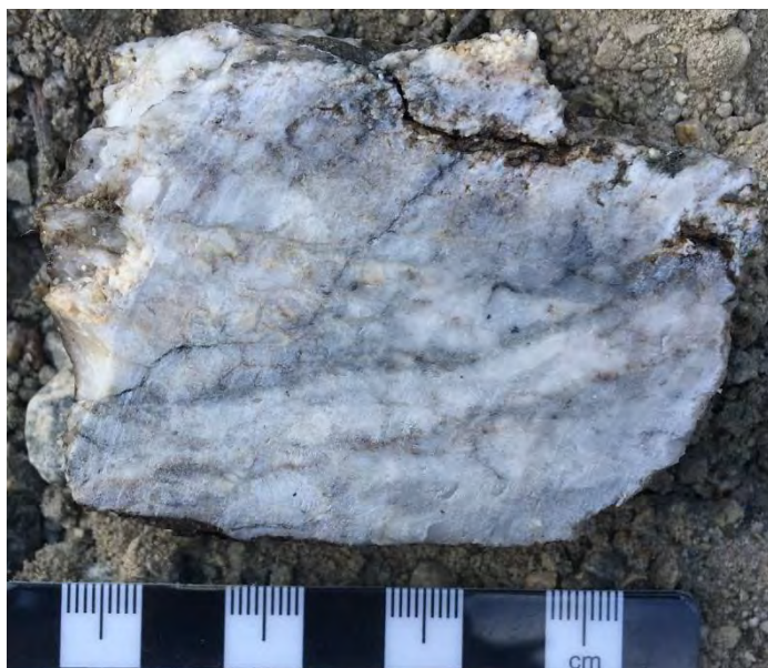
Photo 9.1: GL2 Target Area, EP Zone epithermal mineralization sample no. GLVB18-31R – 18.4 g/t Au, 3,180 g/t Ag. For location of samples see Figure 7.8 & Table 7.4 (A. Albano, 2019)
