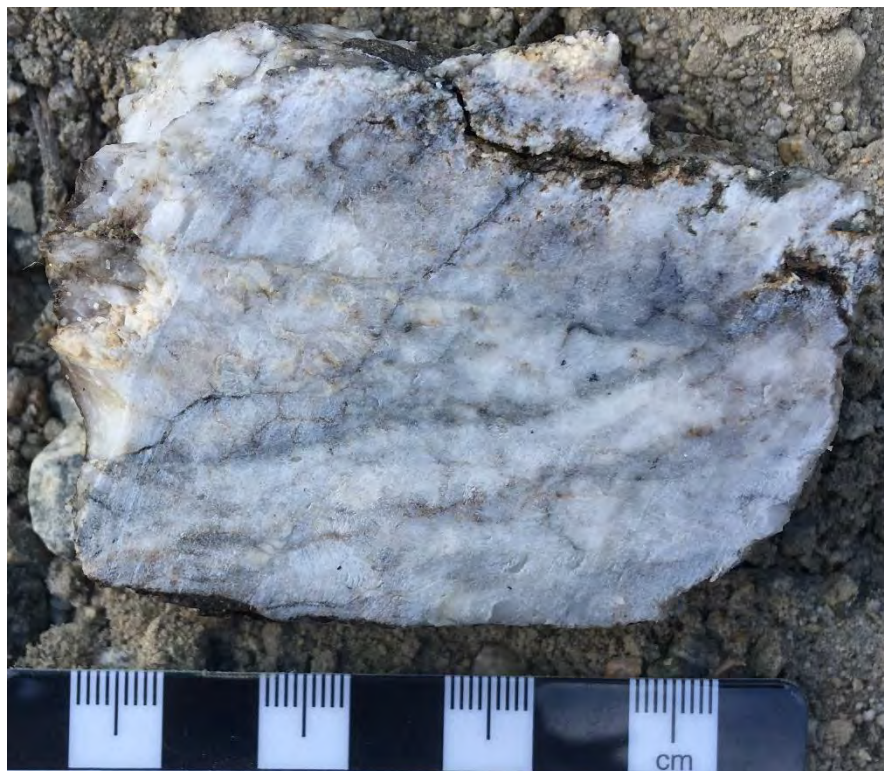
Photo 7.9: GL2 Target Area, EP Zone epithermal mineralization sample no. GLVB18-31R – 18.4 g/t Au, 3,180 g/t Ag. For locations of samples see Figure 7.8 & Table 7.4 (A. Albano, 2019)
