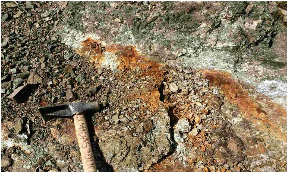
SR-SNO-2016-019 Sediments x-cut by carb+qz vein zone @ 347/15 to NE. strong feox staining locally within veinzone, sulfides are weathered and indistinguishable
