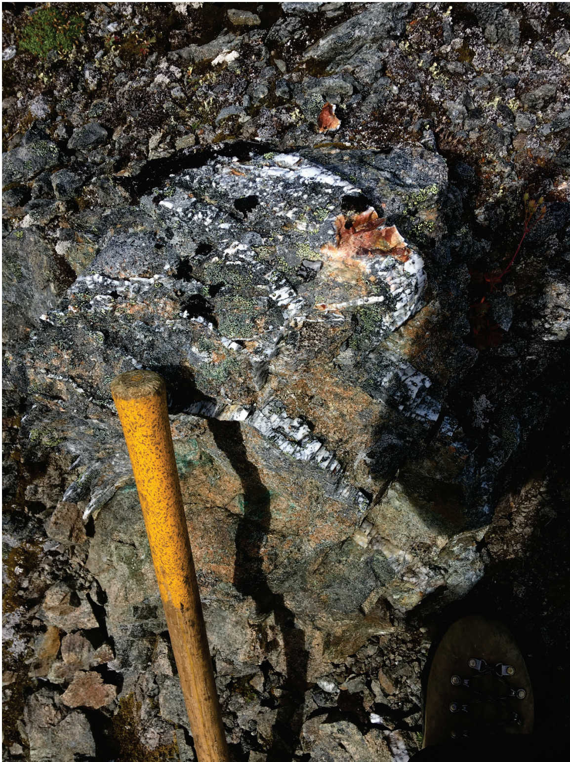
Photo 8.1: Quartz veins containing 2-3% chalcopyrite and abundant malachite staining in a plagioclase porphyry intrusive (sample no. GLAA18-029R (A. Albano, 2018))
