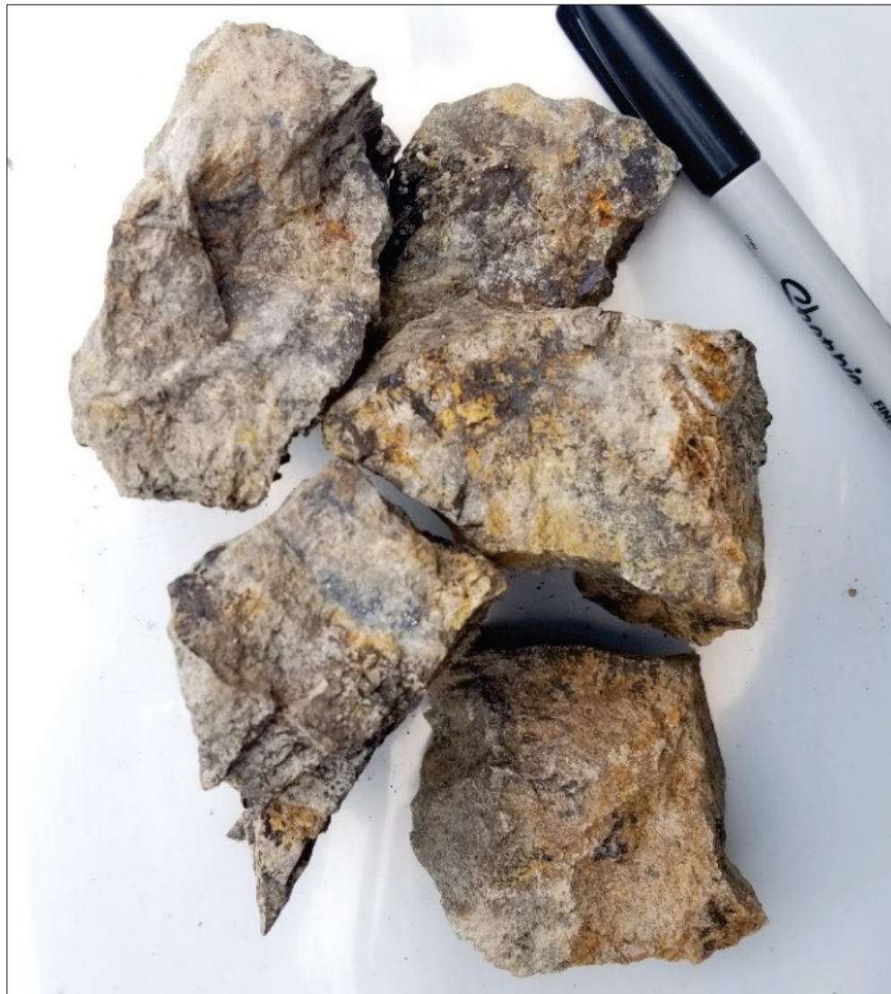
Photo 12.1. Sample T19GL1F-03: Potassic altered felspar intrusive (monzonite?) with boxwork textured quartz veining and minor galena. Dendritic manganese is common on fractures (D. Tupper, 2019)
